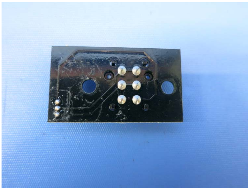
Base Unit Hookswitch PCB solder side
