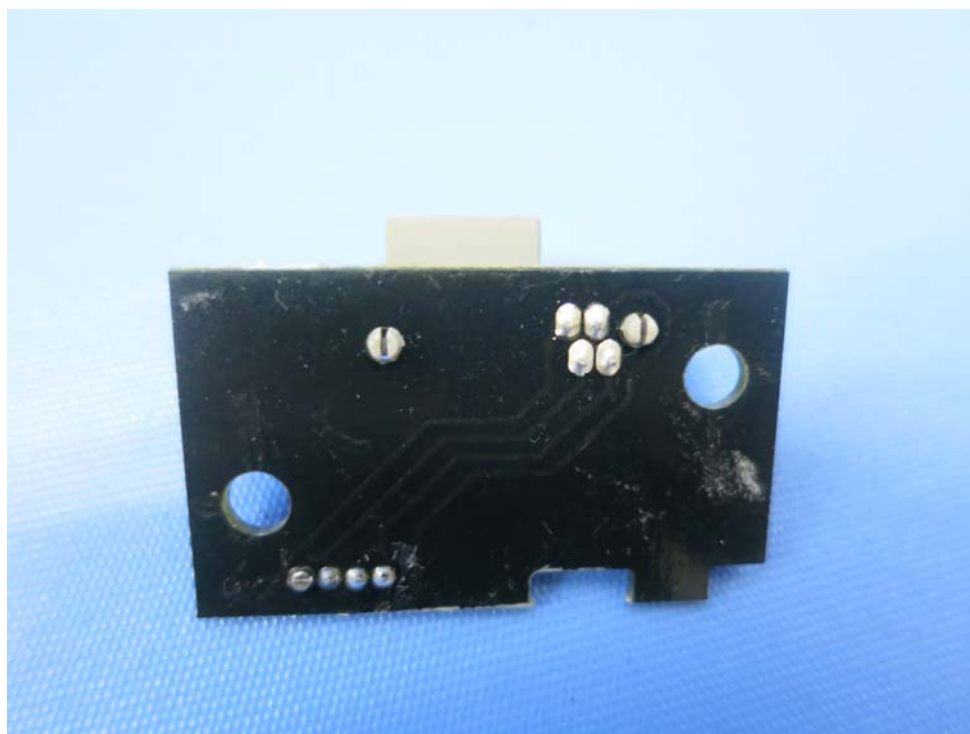
Base Unit modular jack PCB solder side
