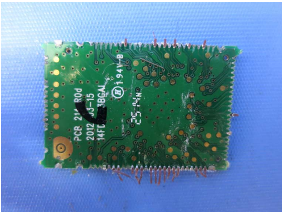
Base Unit Oscillator solder side
