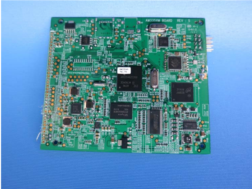
Base Unit AM3354BZCZ100 PCB comp side
