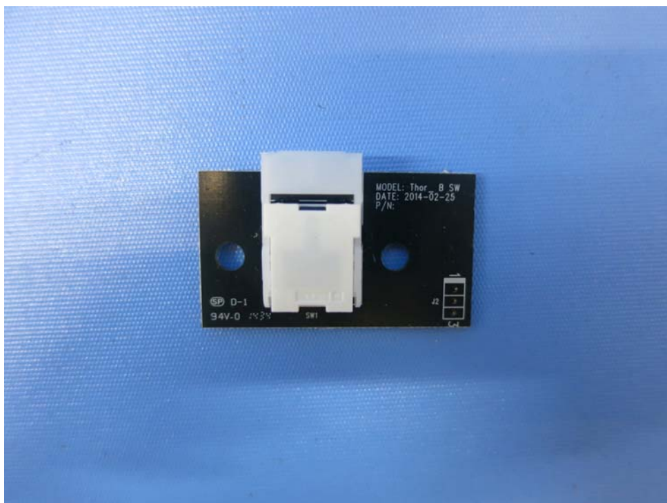
Base Unit Hookswitch PCB comp side
