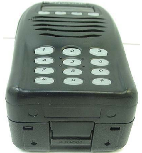
Bottom of DUT with Alkaline Battery Pack
