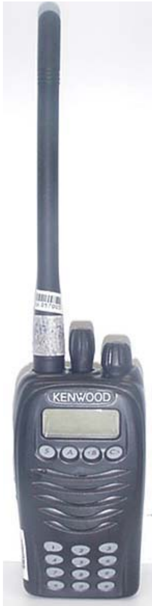
Front of DUT Whip Antenna (P/N: KRA-26M/M2/M3)
