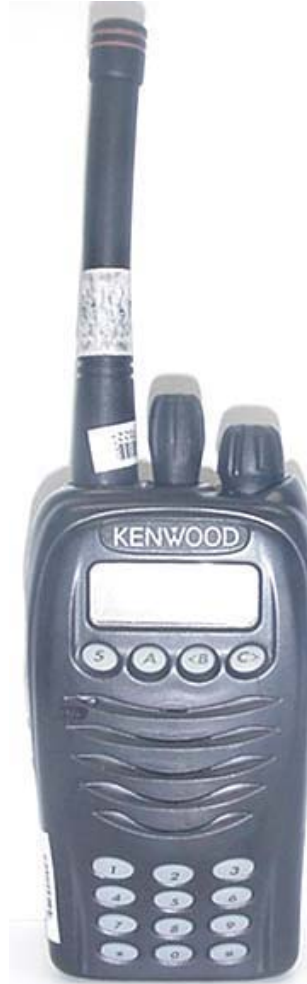
Front of DUT Stubby Antenna (P/N: KRA-16M3)
