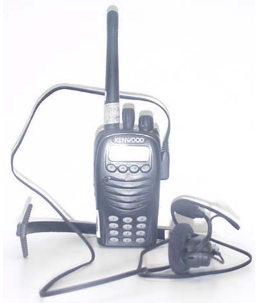
DUT with Boom-Mic Headset Accessory (P/N: KHS-21)
