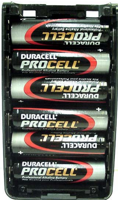
Duracell Procell Alkaline Batteries (Battery Case P/N: KBP-5)
