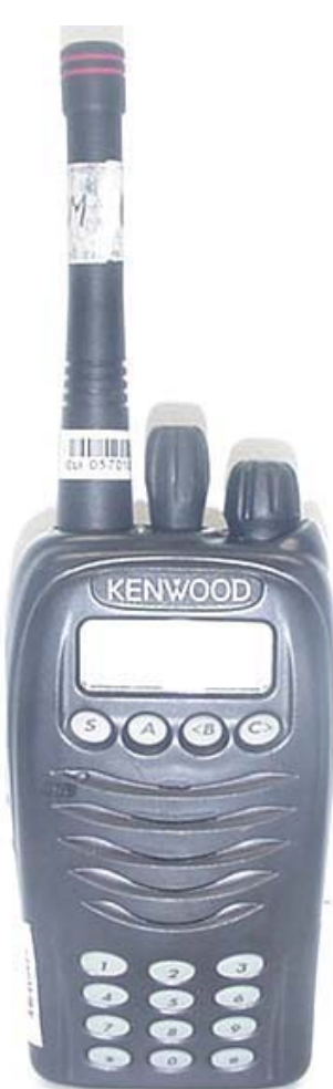
Front of DUT Stubby Antenna (P/N: KRA-16M)
