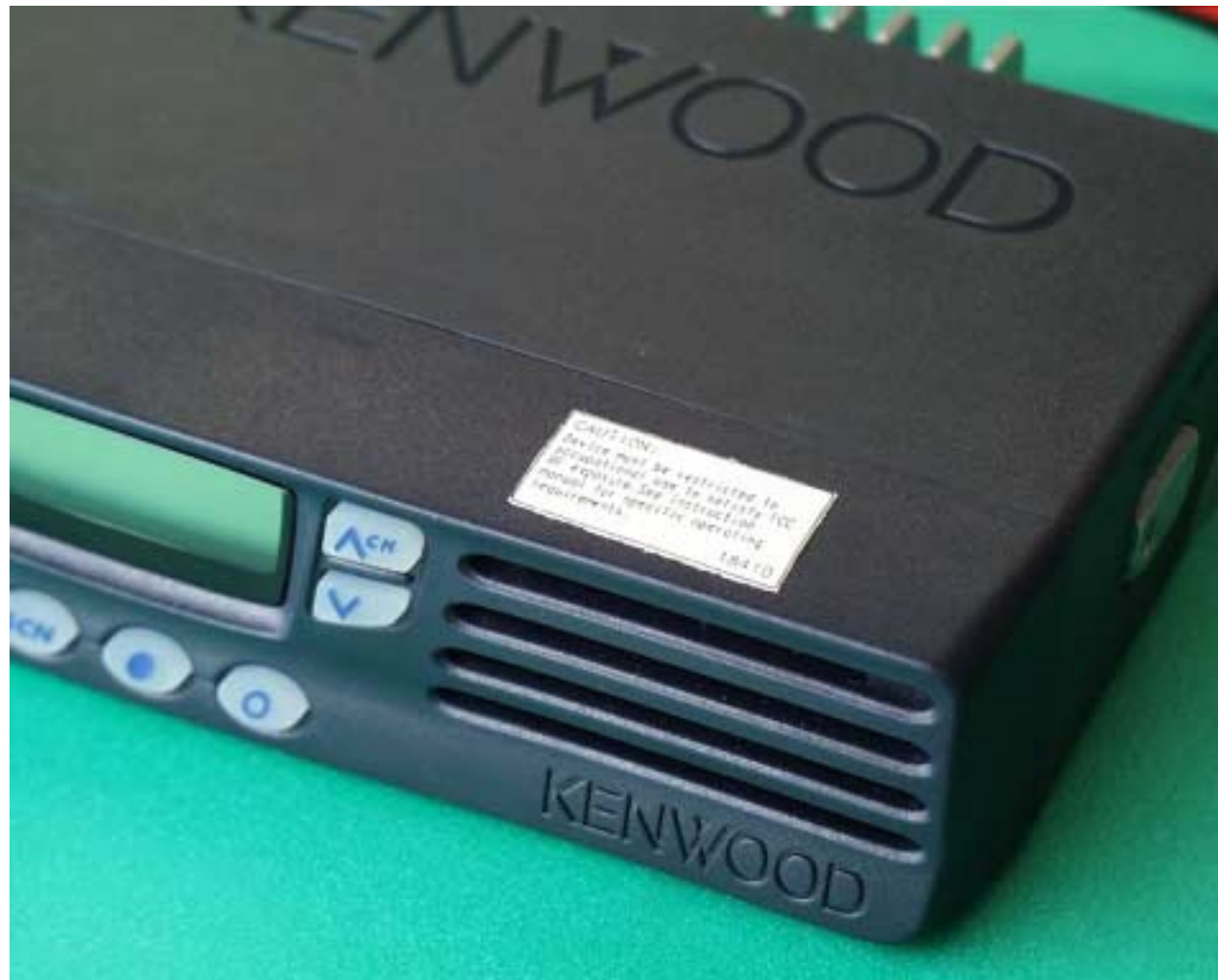
RF EXPOSURE LABEL LOCATION
