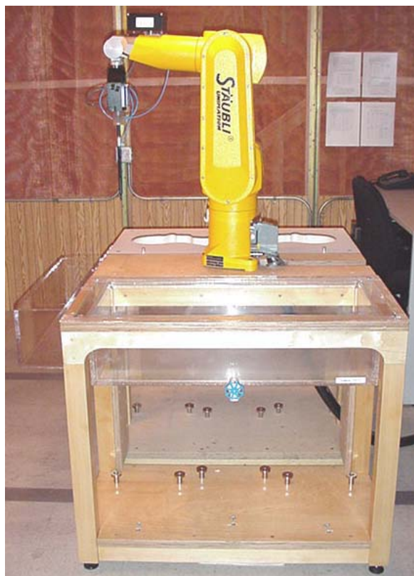
DASY4 SAR Measurement System with validation phantom
