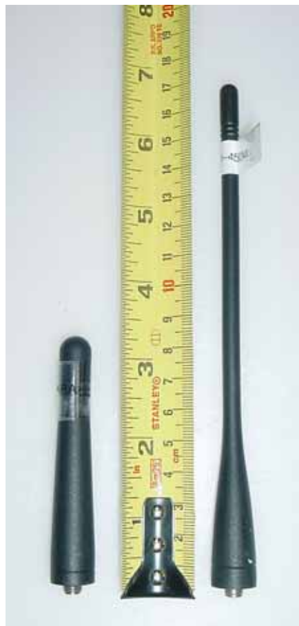
Photograph 18. TK-3202 Whip and Stubby Antennas
