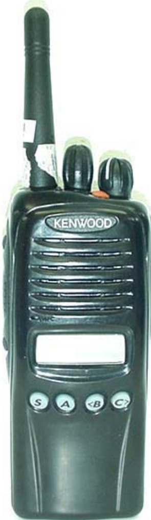
Front of DUT Stubby Antenna (P/N: KRA-23M)
