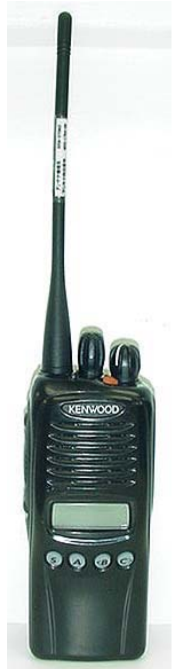
Front of DUT Whip Antenna (P/N: KRA-27M3)
