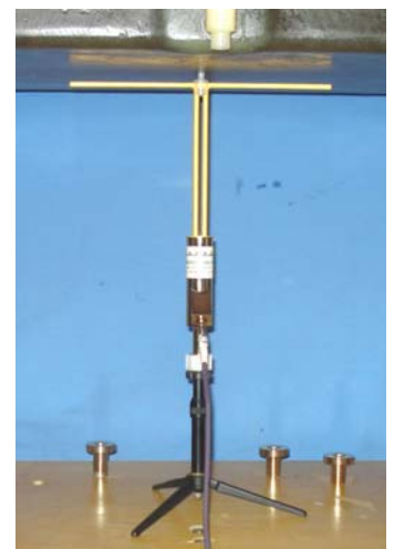
SPEAG 450 MHz Validation Dipole Setup
