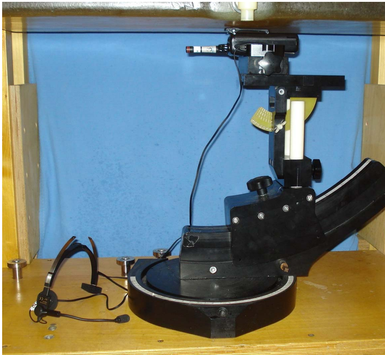
Body-worn SAR Configuration Test Setup
