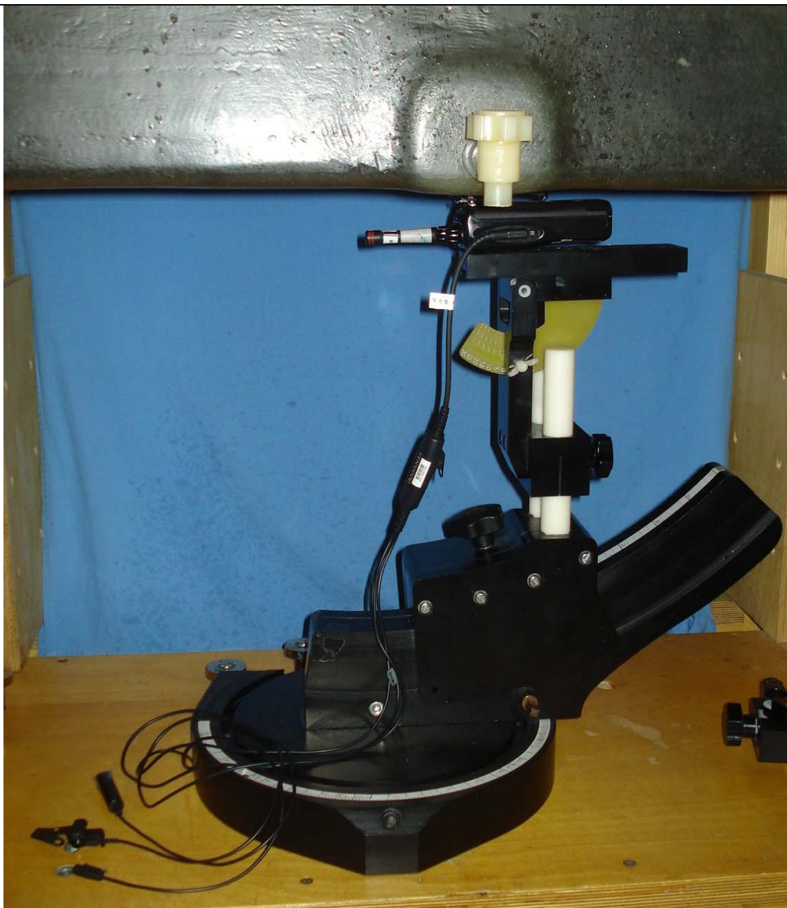
Body-worn SAR Configuration - Antenna 1, Battery a, Audio G5b
