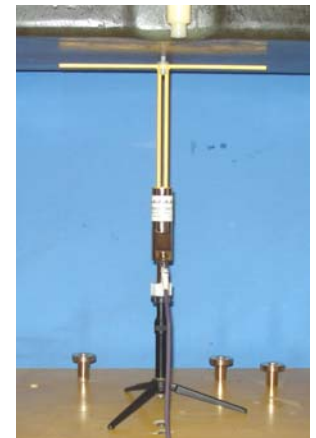
SPEAG 450 MHz Validation Dipole Setup
