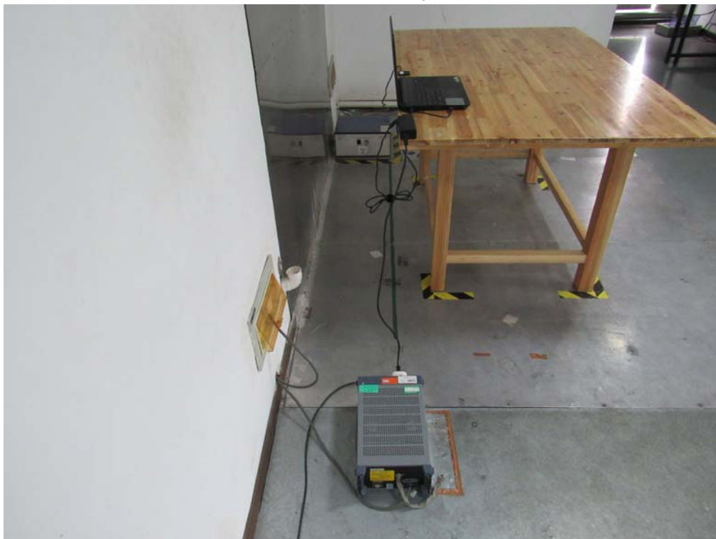
Conducted Emissions Test Setup – Side View
