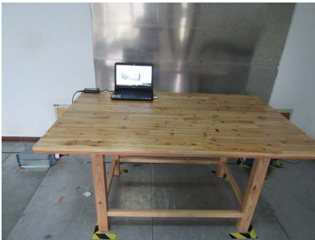
Conducted Emissions Setup Front View
