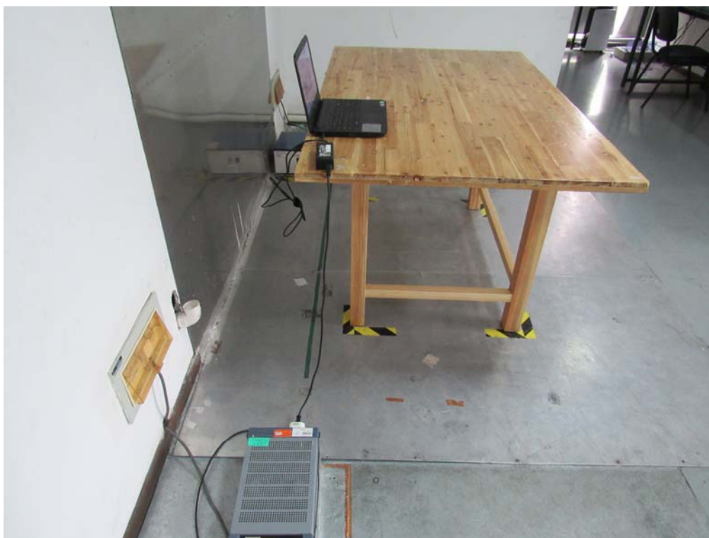
Conducted Emissions Setup Side View
