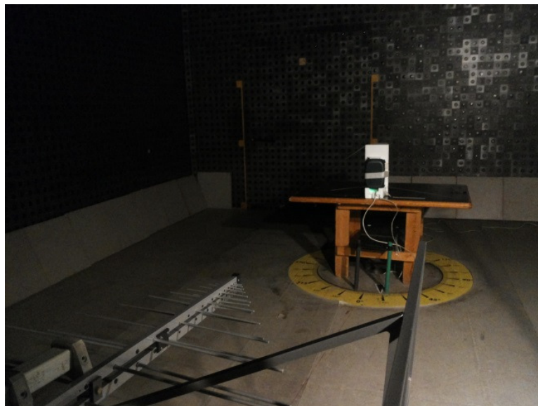
Photograph 8.1.1 Setup for radiated emission measurements
