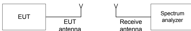
Figure 7.4.1 Occupied bandwidth test setup
