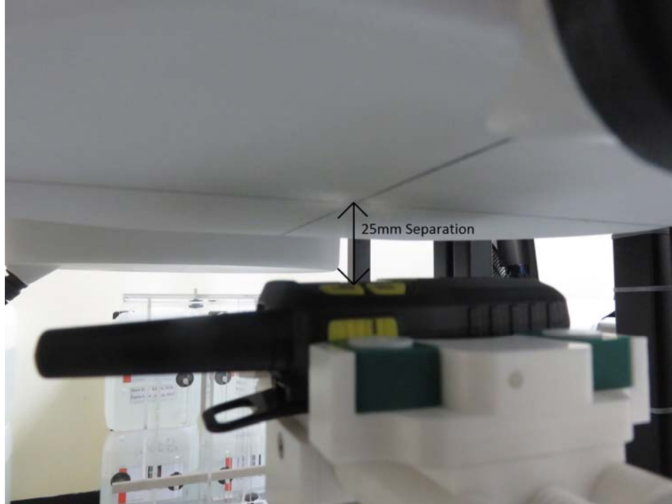
Figure 1 - Front surface with 25mm Separation
