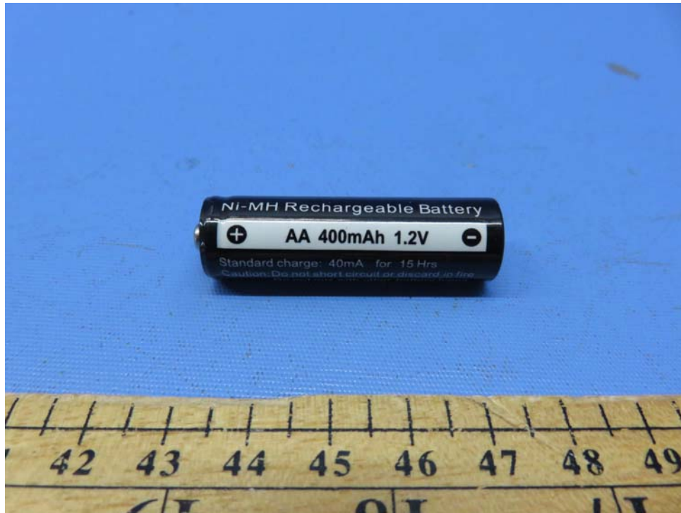
Figure 3 – AA 1.2V 400mAh Ni-MH rechargeable battery
