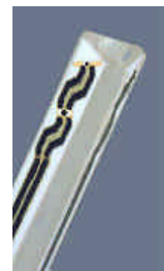
Figure 3.2 Probe Thick-Film Technique
