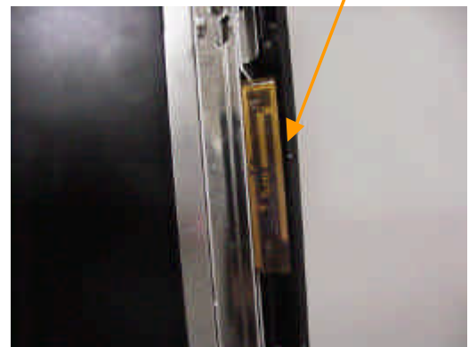
Auxiliary antenna Dual Band Inverted-F type P/N: 3301BZ9077A
