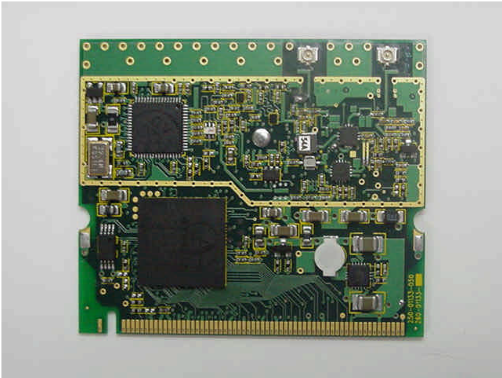
Unshielded Top Side
