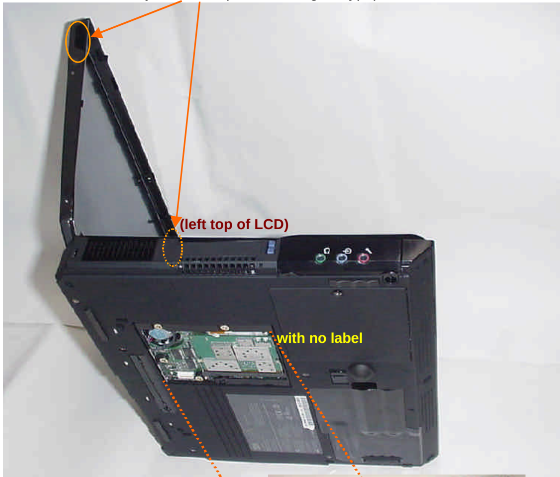
Diversity antennas (inverted F-figure type)
