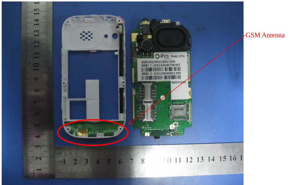
GSM Antenna - Top View
