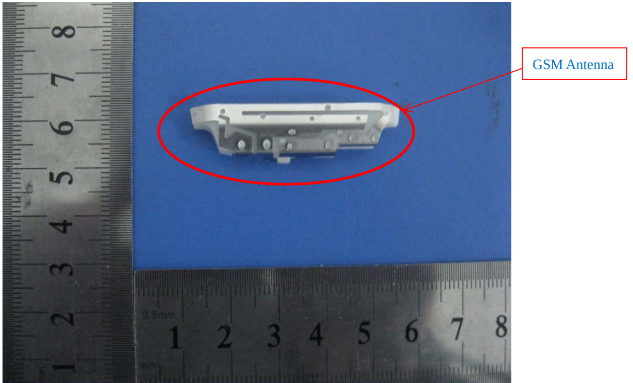
GSM Antenna - Top View
