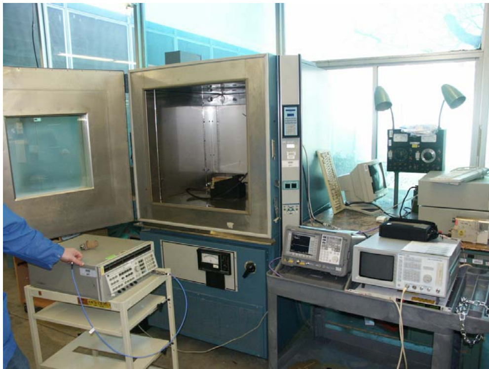
Figure 12-1 Temperature Chamber and Equipment Setup
