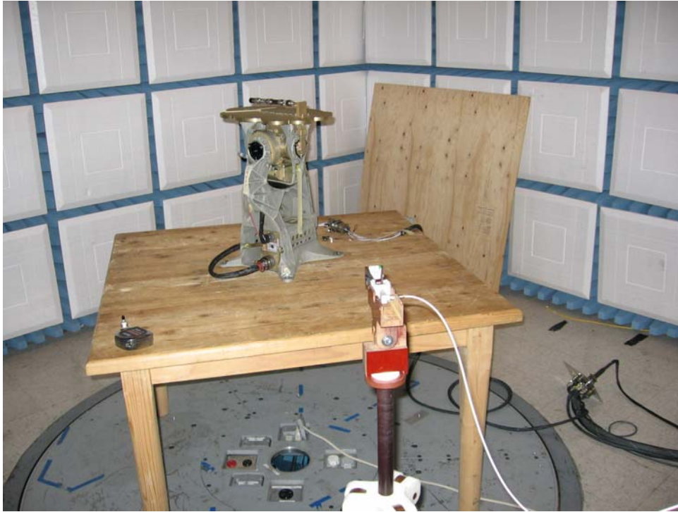
Figure 12-14 Field Strength Measurement 26 – 40 GHz
