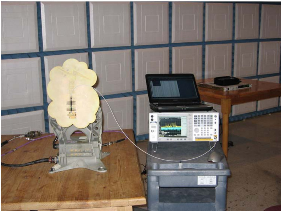
Figure 12-9 Overview Setup and Data Capture of Spurious Emissions at Antenna
