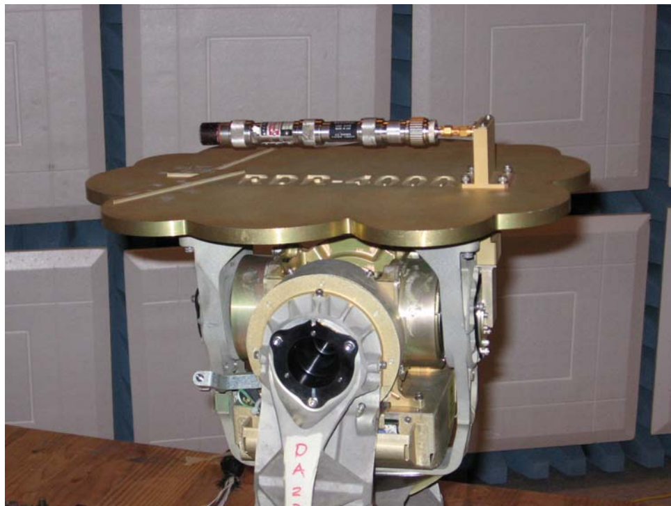
Figure 12-11 Antenna Load for Spurious Emissions – Field Strength
