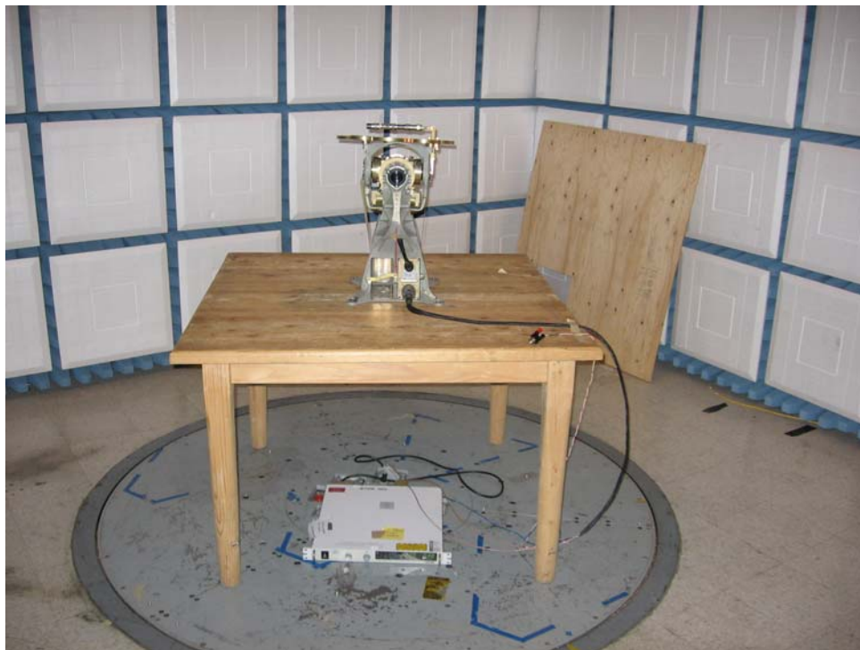
Figure 12-12 Field Strength Measurement 30 MHz – 18 GHz (two antennas)
