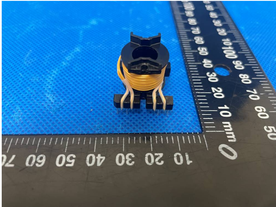
Figure 39. Transformer T901 view 11
