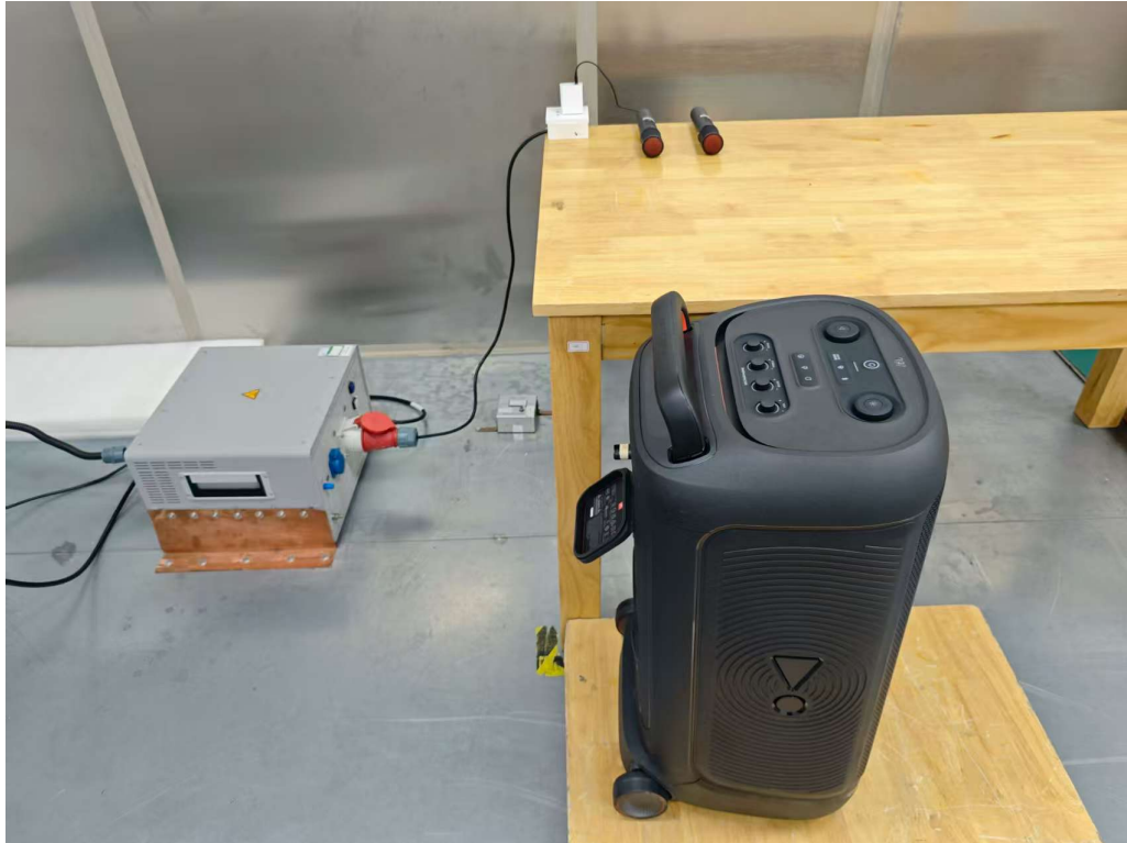
Photograph 3: Set-up for Conducted Emission on AC Mains
