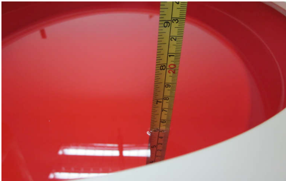
Figure 4.4: Liquid depth in the Flat Phantom
