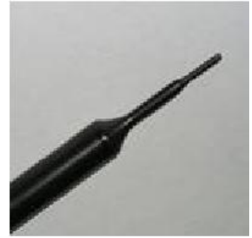
Figure 4.4 EX3DV4 E-field Probe
