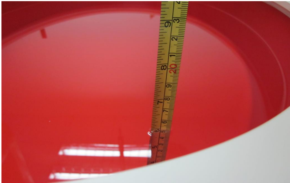
Figure 4.4: Liquid depth in the Flat Phantom
