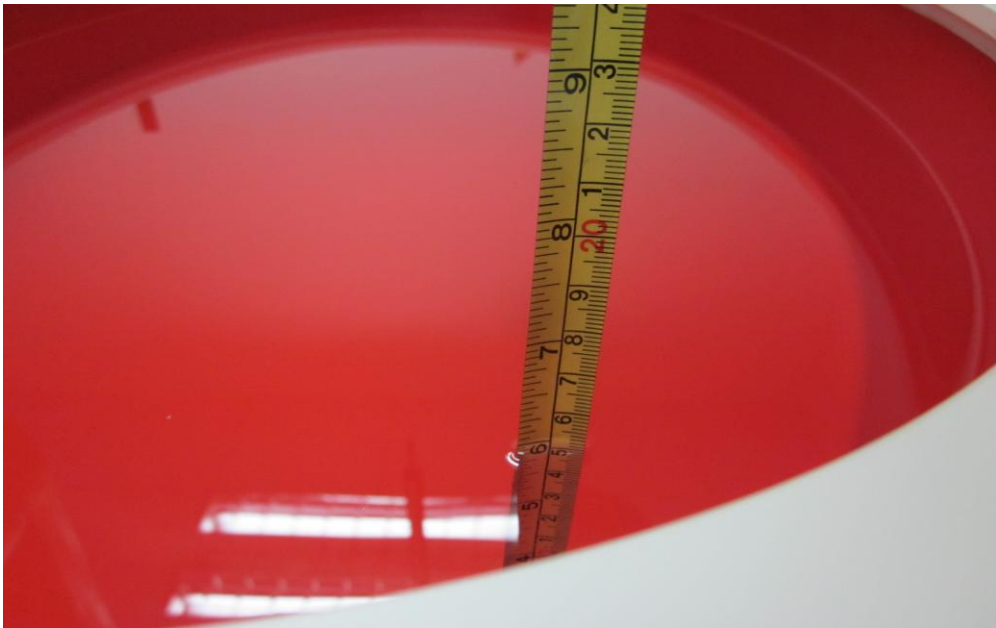
Figure 4.4: Liquid depth in the Flat Phantom
