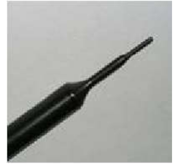
Figure 4.4 EX3DV4 E-field Probe
