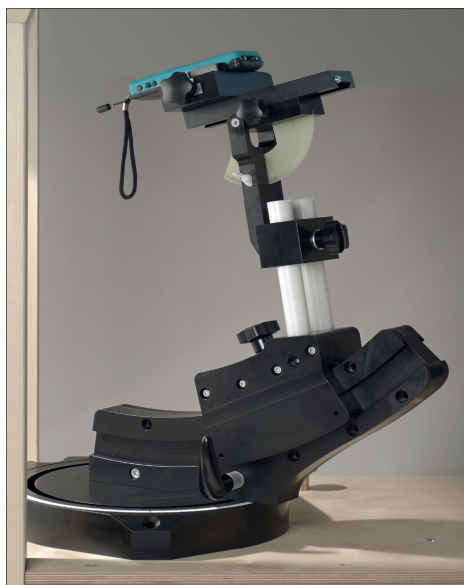
F-2. Device Holder for Transmitters
