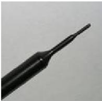
Figure 4.4 EX3DV4 E-field Probe
