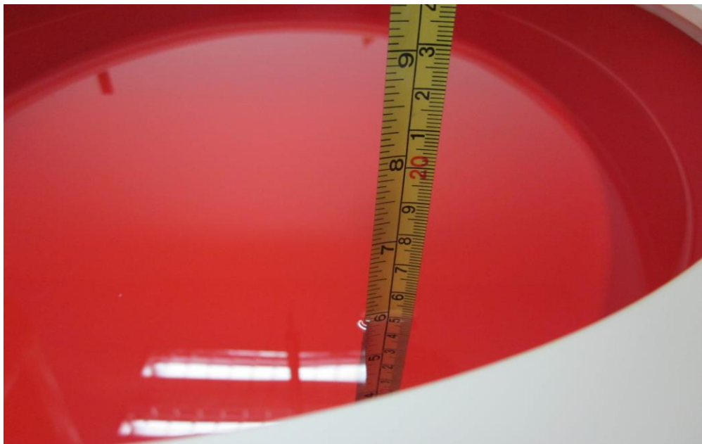
Figure 4.4: Liquid depth in the Flat Phantom
