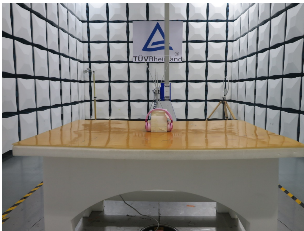
Photograph 1: Set-up for Radiated Spurious Emission, Below 1GHz
