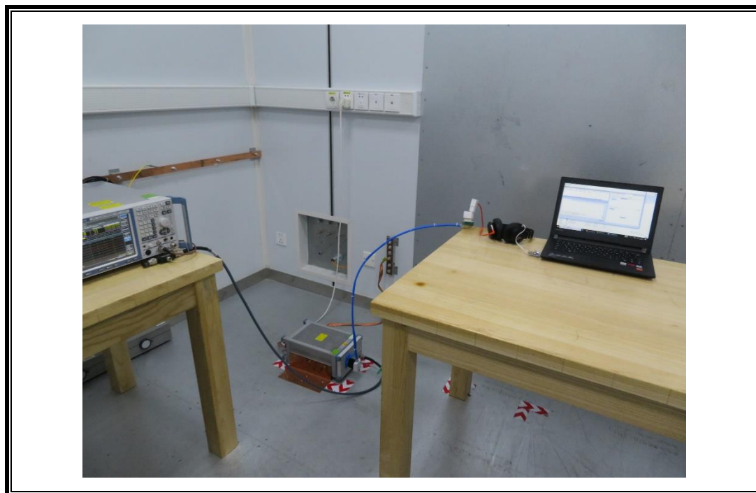
POWERLINE CONDUCTED EMISSIONS MEASUREMENT SETUP
