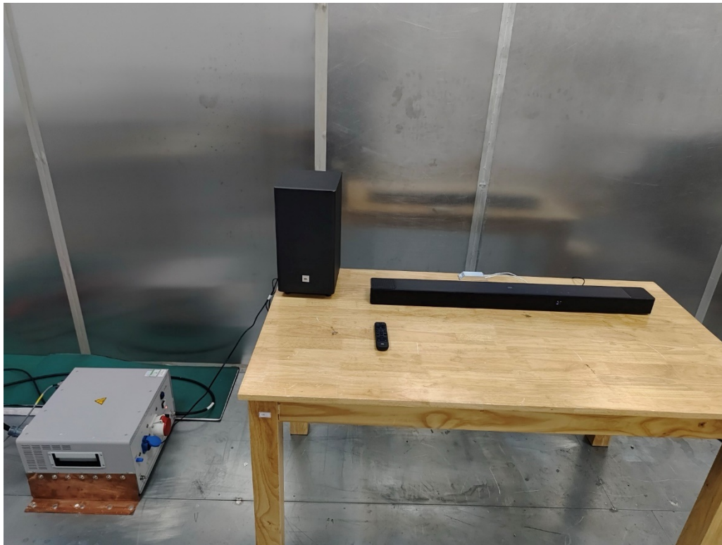
Photograph 3: Set-up for Conducted Emission
