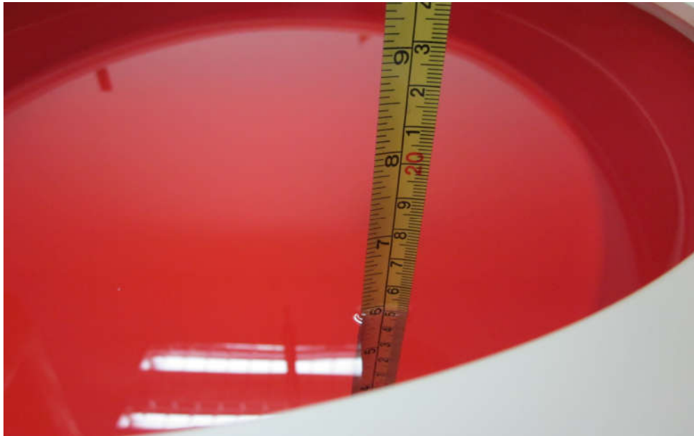
Figure 4.4: Liquid depth in the Flat Phantom
