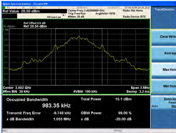
20dB Bandwidth plot on channel 39 (1Mbps)
