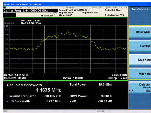
20dB Bandwidth plot on channel 78 (2Mbps)
