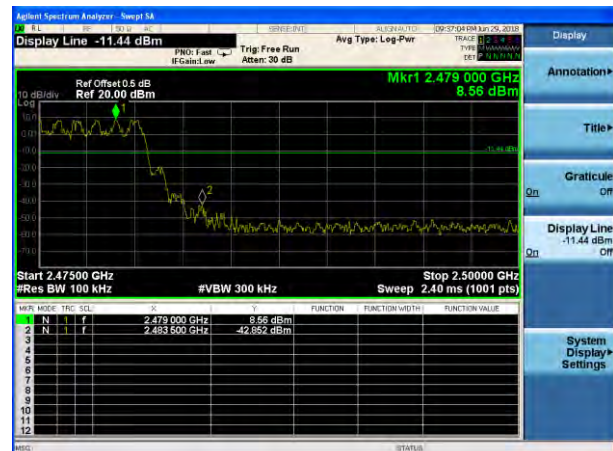
8-DPSK: Band Edge-High Channel (Hopping Mode)
