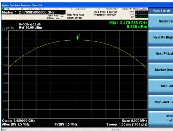
Peak output Power plot on channel 78 (1Mbps)
