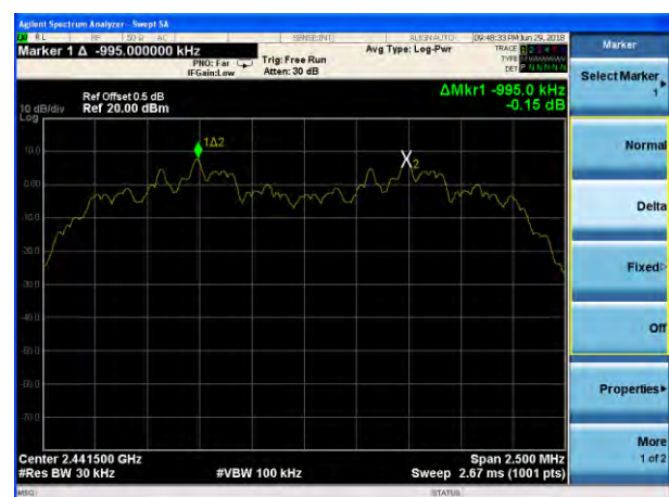
(2Mbps) Channel Separation plot on channel 39-40
