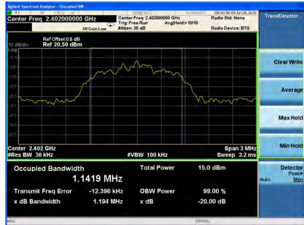
20dB Bandwidth plot on channel 39 (2Mbps)
