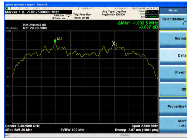
(2Mbps) Channel Separation plot on channel 39-40
