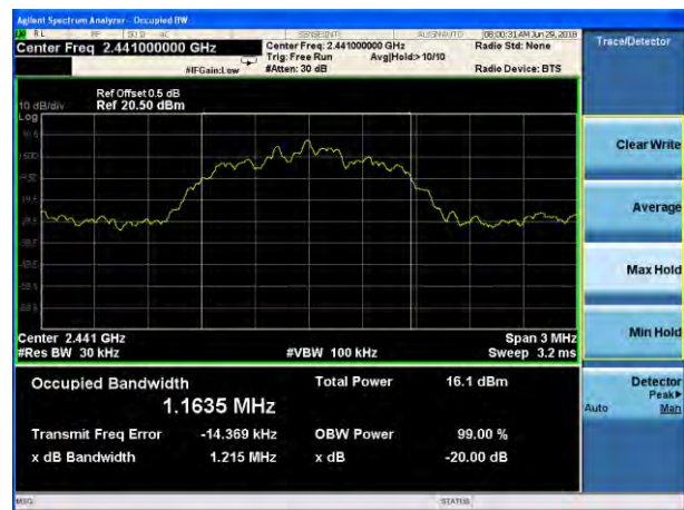
20dB Bandwidth plot on channel 78 (2Mbps)
