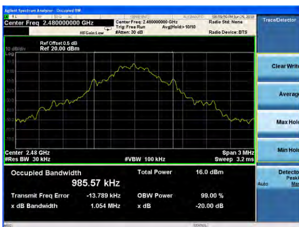
20dB Bandwidth plot on channel 78 (1Mbps)
