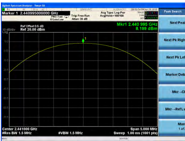
Peak output Power plot on channel 39 (1Mbps)
