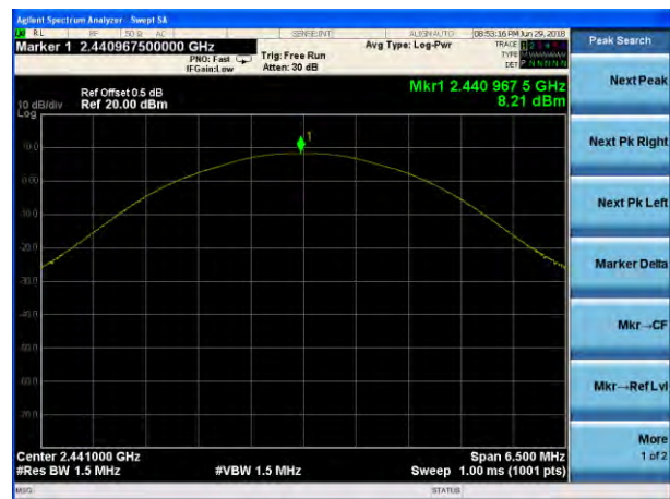
Peak output Power plot on channel 39 (2Mbps)
