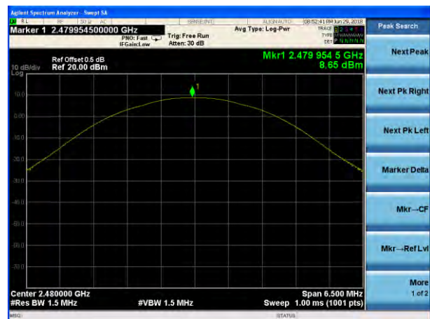
Peak output Power plot on channel 78 (2Mbps)
