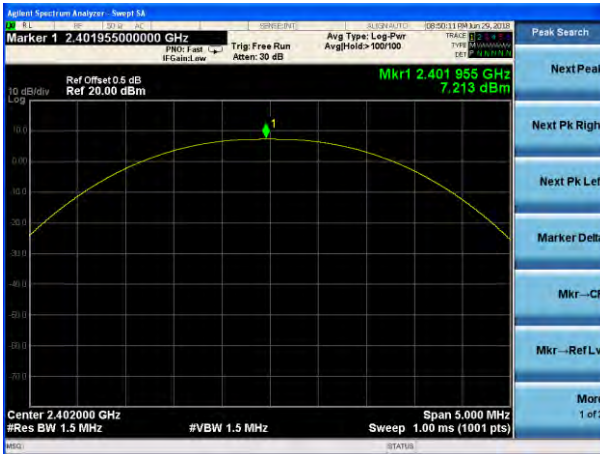
Peak output Power plot on channel 39 (1Mbps)
