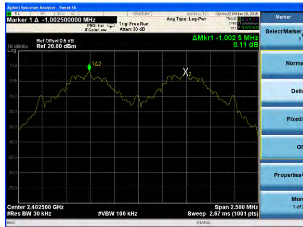
(1Mbps) Channel Separation plot on channel 39-40
