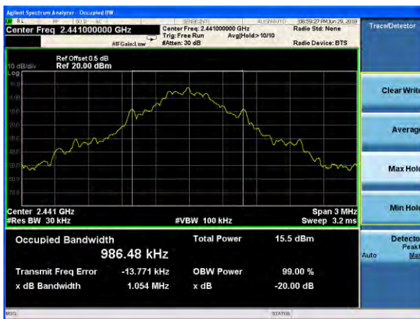
20dB Bandwidth plot on channel 78 (1Mbps)
