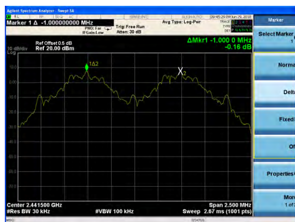
(1Mbps) Channel Separation plot on channel 39-40
