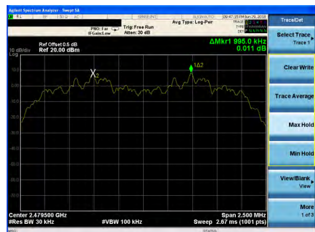
(2Mbps) Channel Separation plot on channel 77-78
