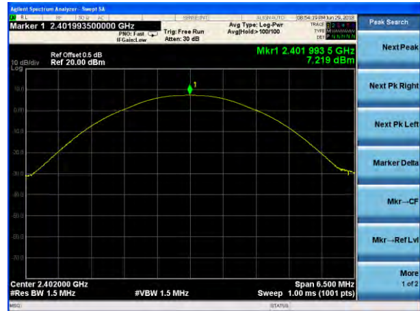
Peak output Power plot on channel 39 (2Mbps)
