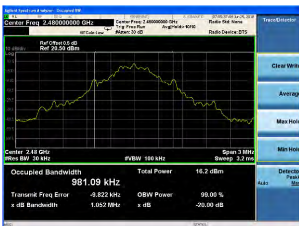
20dB Bandwidth plot on channel 78 (1Mbps)
