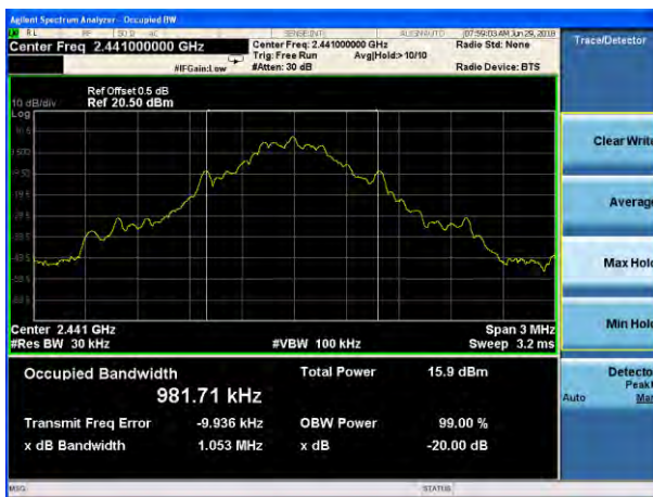
20dB Bandwidth plot on channel 78 (1Mbps)
