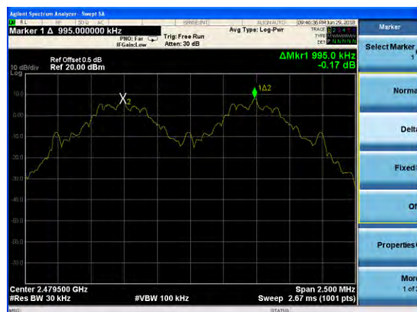
(1Mbps) Channel Separation plot on channel 77-78
