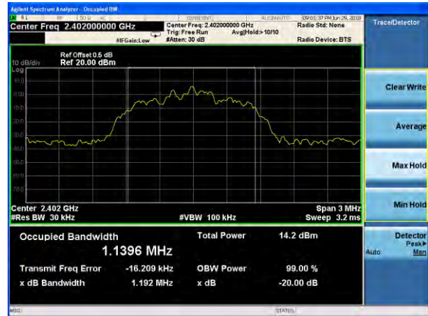
20dB Bandwidth plot on channel 39 (2Mbps)
