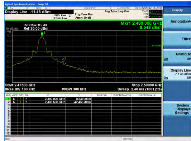
8-DPSK: Band Edge-High Channel
