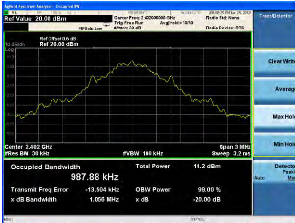
20dB Bandwidth plot on channel 39 (1Mbps)
