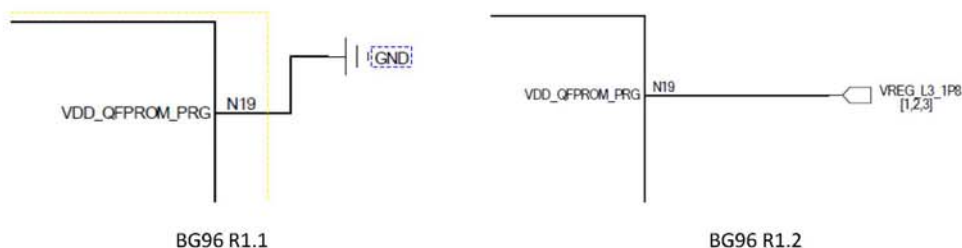
Figure 1: Schematic Designs of BG96 R1.1 and R1.2
