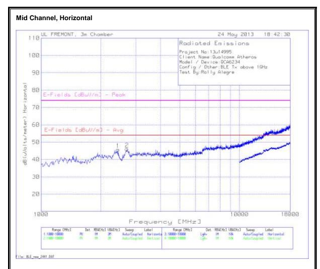
**Note:** No other signals were detected above system noise floor level up to 26 GHz.
