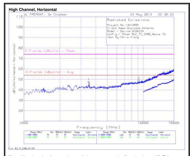
Note: No other signals were detected above system noise floor level up to 26 GHz.
