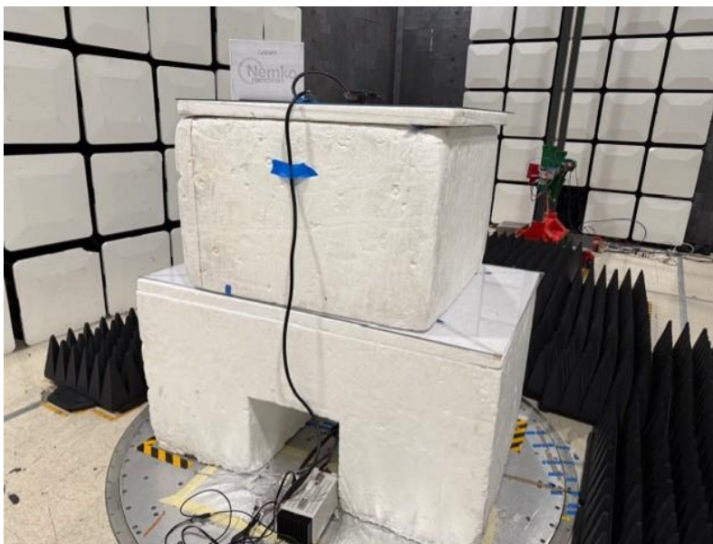
Figure 8.1-3: Radiated emissions setup for Bluetooth band edge test (rear view)
