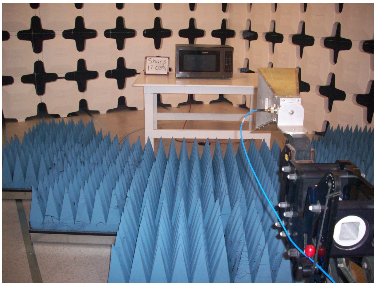
Figure 4. Radiated Emissions Measurement Photo, above 1000 MHz
