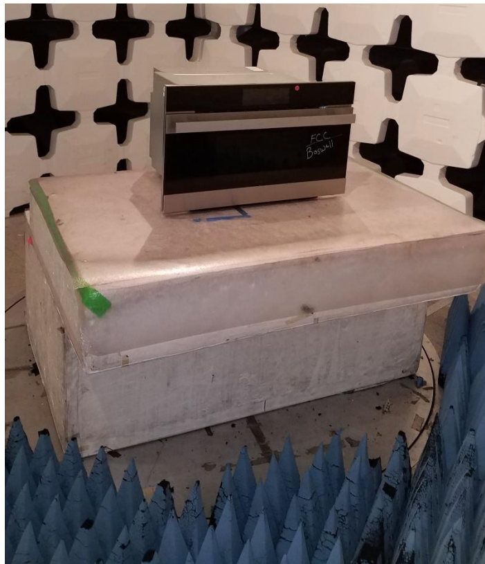
Figure 12. Photograph of Radiated Emissions Test Configuration, Close-Up
