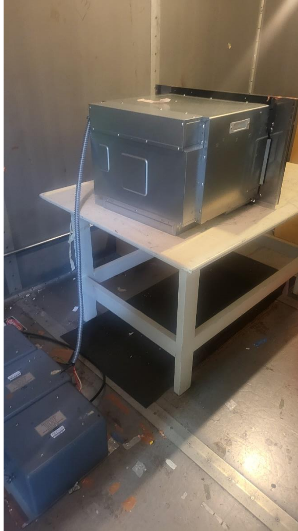
Figure 11. Photograph of Conducted Emissions Test Configuration
