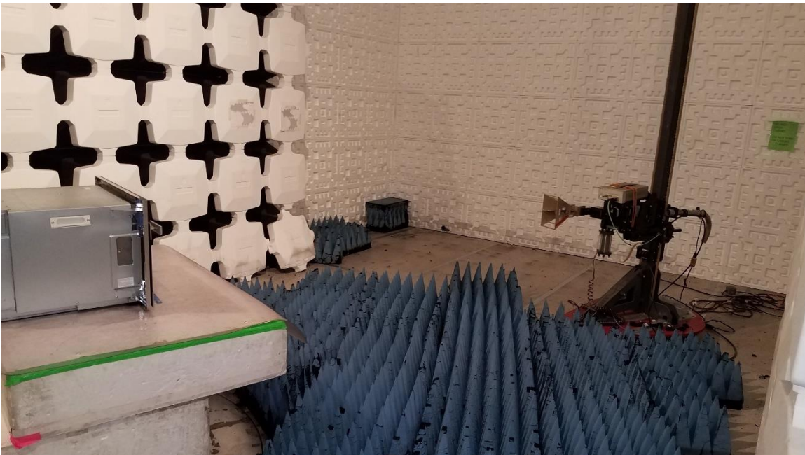
Figure 15. Photograph of Radiated Emissions Test Configuration, 1 - 25 GHz
