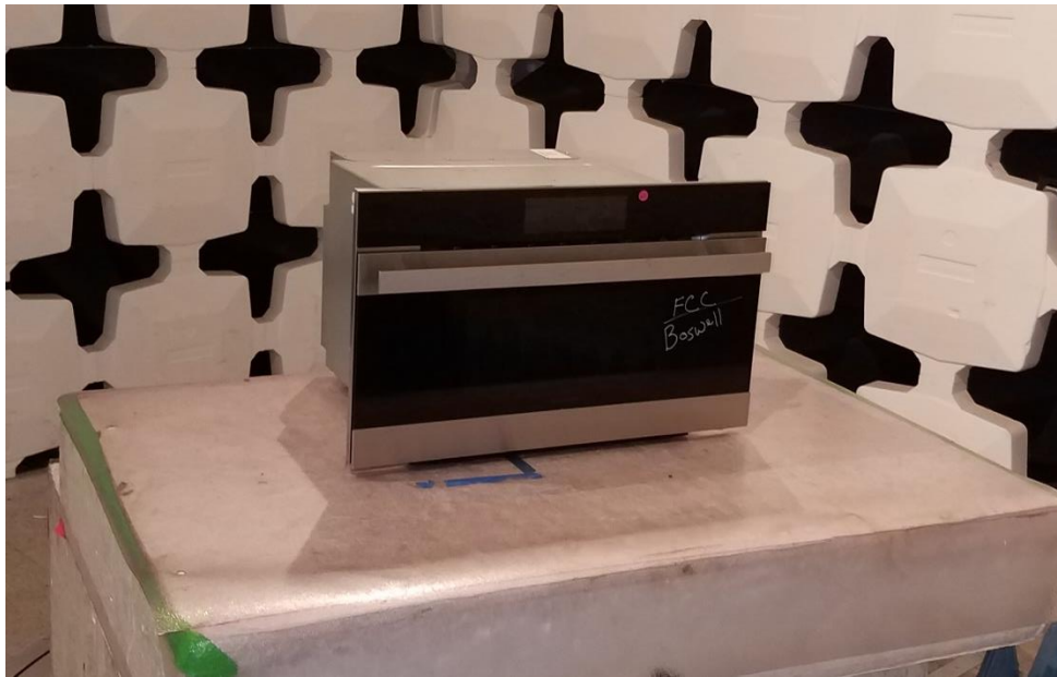
Figure 1. Radiated Emissions Measurement Photo (Front View)
