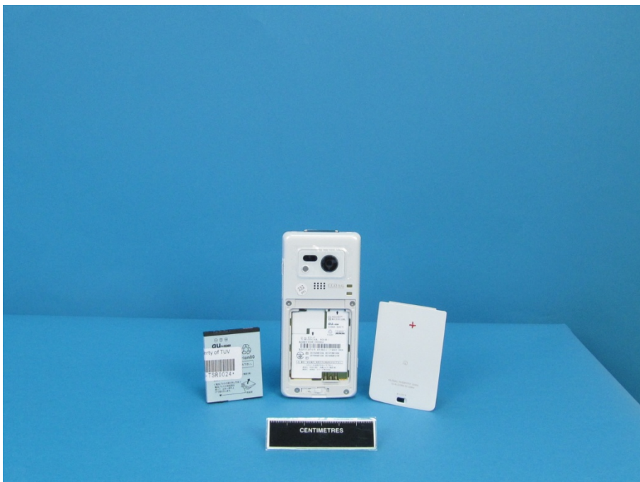
Figure 23 Rear View – SH011 Battery Removed
