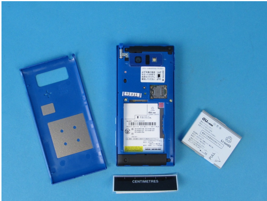
Figure 30 Rear View Battery Removed (CDMA 2000)
