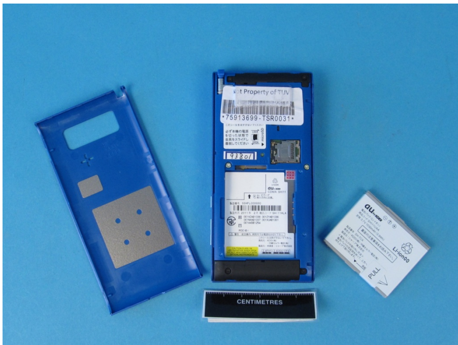
Figure 31 Rear View Battery Removed (WLAN)
