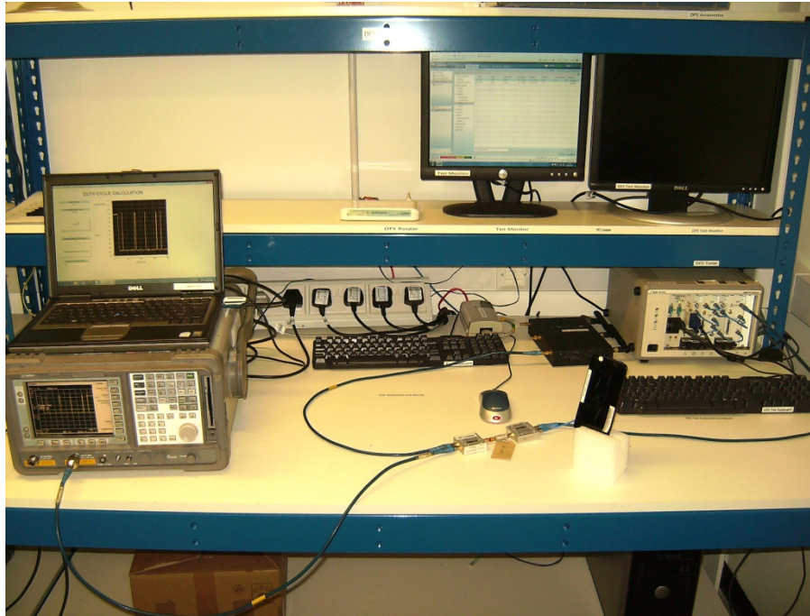
DFS Testing – Duty Cycle Set-Up
