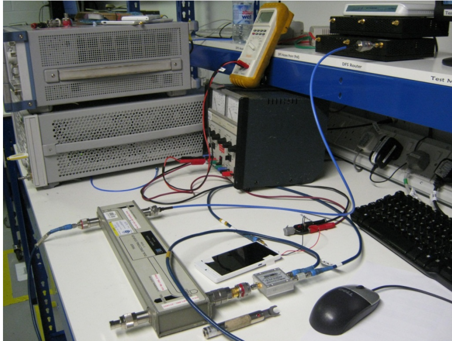
DFS - Testing Set-Up
