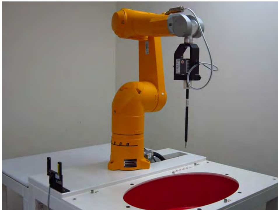
Fig.1 Photograph of the SAR measurement system
