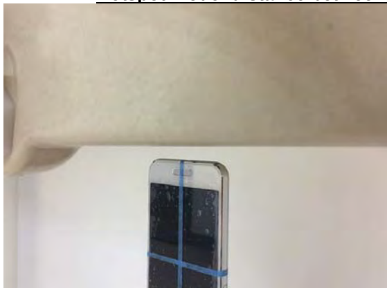
Fig.12 EUT Bottom side to flat phantom
