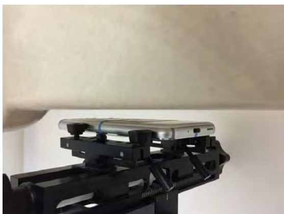
Fig.8 EUT Back side to flat phantom
