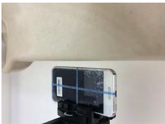
Fig.13 EUT Right side to flat phantom
