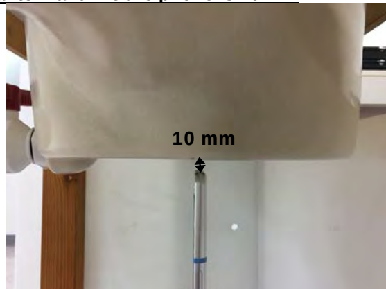
Fig.12 EUT Bottom side to flat phantom
