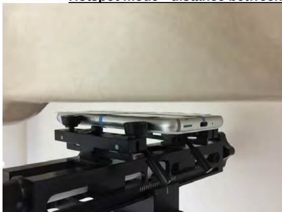
Fig.9 EUT Front side to flat phantom
