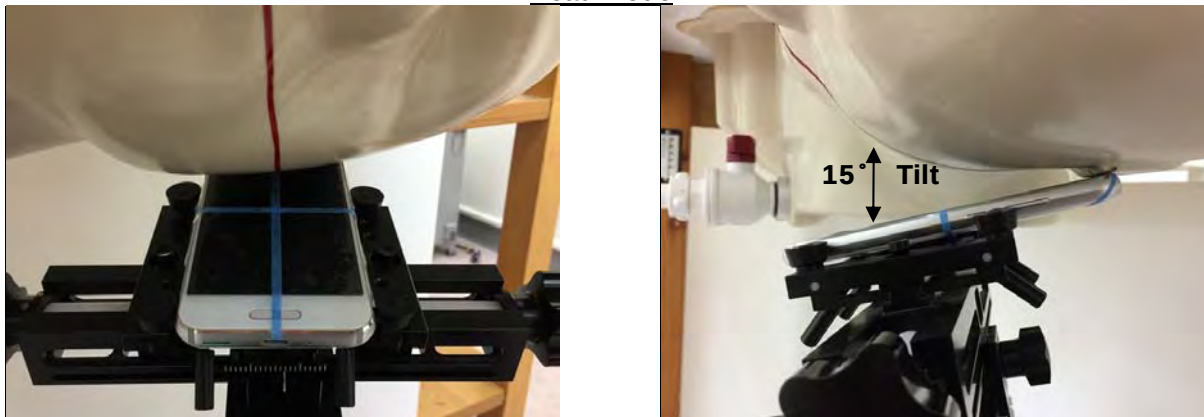
Fig.6 Left Head Section / Ear-Tilt Position(15°)
