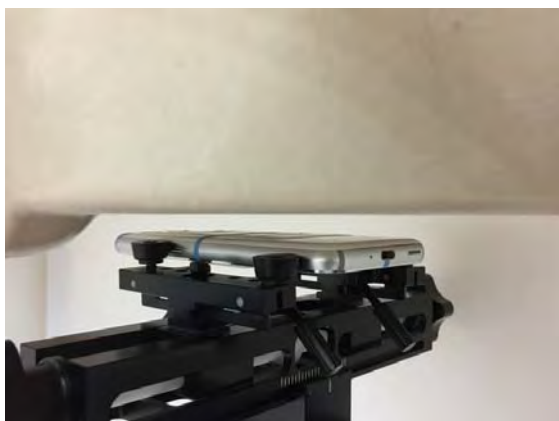
Fig.10 EUT Back side to flat phantom
