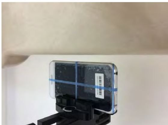
Fig.14 EUT Left side to flat phantom
