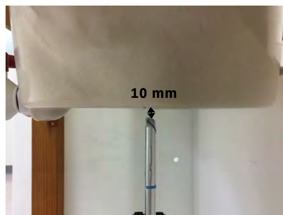
Fig.11 EUT Top side to flat phantom
