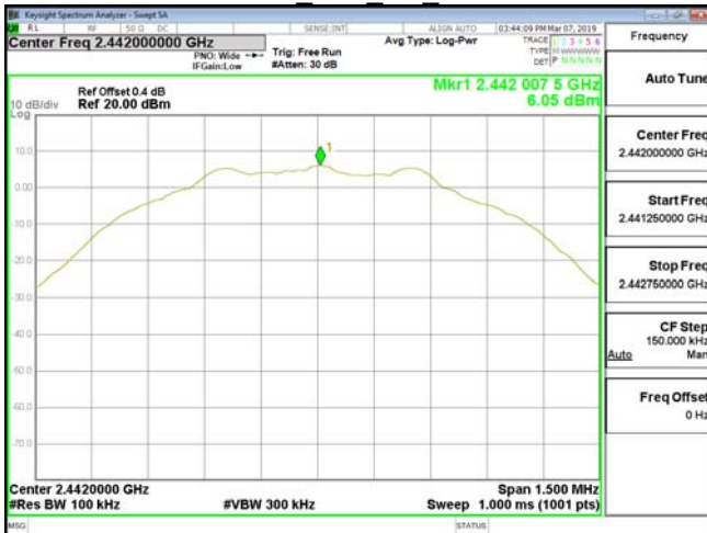
Reference Level BLE 1M HighCH39-2480
