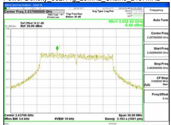
Power Density 802.11g 20MHz Chain0 2462MHz
